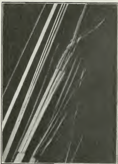
Break in fibre from the Pilbarra district, Western Australia. Magnified 150 diameters.
